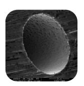
The PSA DW10B engine (4 cylinders, common rail direct injection, 2.0L displacement) is used to evaluate the propensity of diesel fuel or diesel additives to prevent deposits formation in injector nozzles. The engine is operated for 16 hours with blank DF-79 fuel, then for 56 hours with the additive (including 3\*8 hours of engine stop). The propensity of the fuel to promote deposits formation in the nozzles is determined by measuring the power change between start-of-test and end-of-test.
