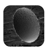
The PSA DW10B engine (4 cylinders, common rail direct injection, 2.0L displacement) is used to evaluate the propensity of diesel fuel or diesel additives to prevent deposits formation in injector nozzles. The engine is operated for 16 hours with blank DF-79 fuel, then for 56 hours with the additive (including 3\*8 hours of engine stop). The propensity of the fuel to promote deposits formation in the nozzles is determined by measuring the power change between start-of-test and end-of-test.
