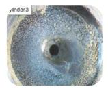
The PSA XUD9 engine (4 cylinders, <u>indirect injection</u>, 1.9L displacement) is used to evaluate the propensity of diesel fuel and diesel additives to prevent deposits formation in injector nozzles. The engine is operated at low speed/load for a period of 10 hours. XUD9 is a worldwide reference test for diesel fuel quality.
