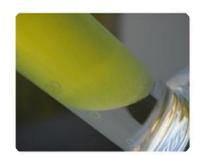
This test consists of agitating for 2 minutes a 80/20 mL blend of diesel fuel and water and observing both rapidity and quality of phase separations. The purpose of the test is to see if the additized diesel fuel can easily separate water, in case of any ingress during transportation and handling.
