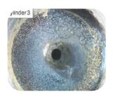
The PSA XUD9 engine (4 cylinders, <u>indirect injection</u>, 1.9L displacement) is used to evaluate the propensity of diesel fuel and diesel additives to prevent deposits formation in injector nozzles. The engine is operated at low speed/load for a period of 10 hours. XUD9 is a worldwide reference test for diesel fuel quality.
