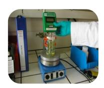
For security reasons (electrostatic discharge during fuel transportation or transfer), specifications might be set on electrical conductivity of road fuels. ASTM D-2624 method allows to determine the conductivity of the liquid fuels by dipping the electrode in the sample of fuel.
